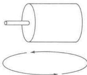
Here, a generalized unstable satellite (A) begins to nutate, (B) rapidly increases its 'coning' movement, (C) enters a flat spin. Between 'A' and 'C', all the spin about the long axis has changed to lateral spin. Try this out with a child's top.
