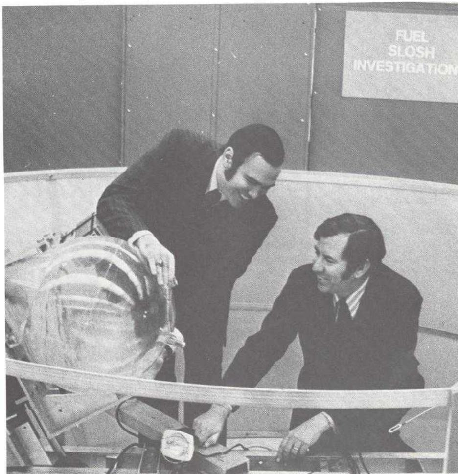
Ernesto R. Martin, principal COMSAT investigator for the project, and James R. Owens, manager of the positioning and orientation branch, COMSAT Labs, with the spinning device used to simulate the sloshing of fuel on INTELSAT IV.
