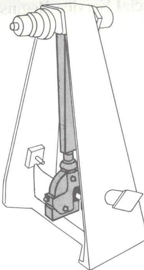
An actual nutation damper for INTELSAT IV. The dark area is the pendulum arm. The device is open, just as you see it here.
