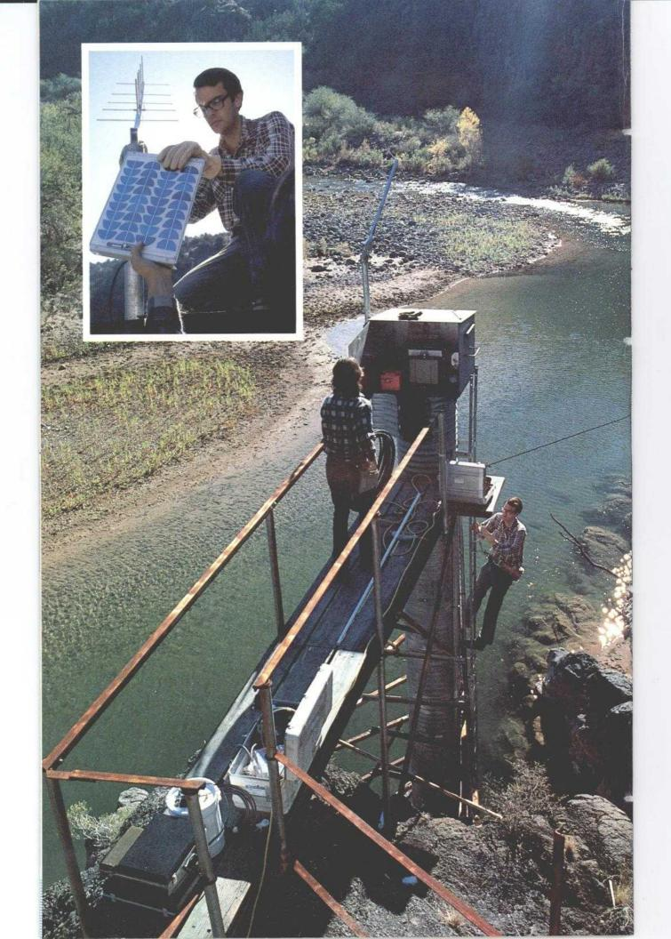
An employee of USGS or a cooperating organization hikes, takes four-wheel-drive vehicle or helicopter to the station, enters it, and either writes down the information shown or collects the paper tape from the water height recorder inside. After he reaches civilization, the data is then transmitted to Reston over phone lines.
