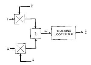
Figure 10. Generalized Tracking Loop Processing
