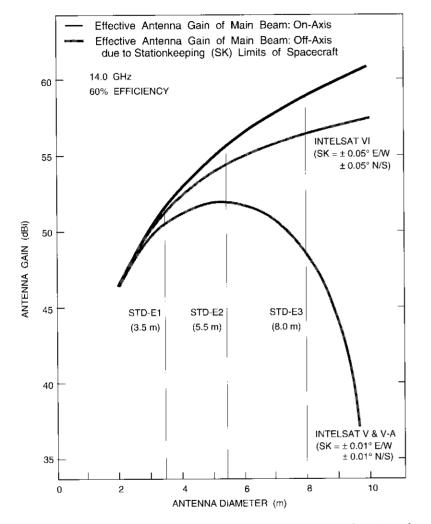
Figure 1. On- and Off-Axis Main Beam Antenna Gain as a Function of Earth Station Antenna Size and Satellite Stationkeeping Tolerance (Ku-band, fixed antennas)
