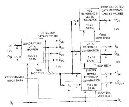
Figure 9. Quadrature Channel Detection and Data Feedback Mappings
