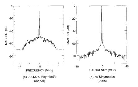
Figure 28. Symbol Timing Tracking Loop Output Phase Noise
