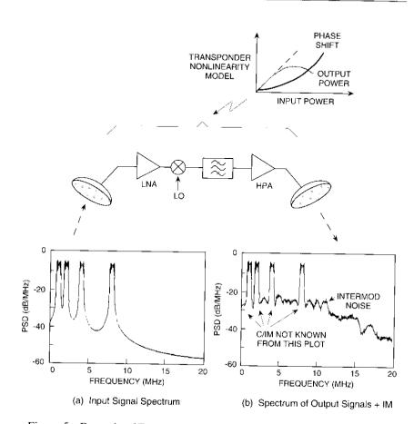
Figure 5. Example of Transponder Loading With Equal Amplitude Signals and 3rd-Order IM-Free Spacing
