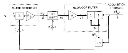
Figure 12. Symbol Timing Tracking Loop Model
