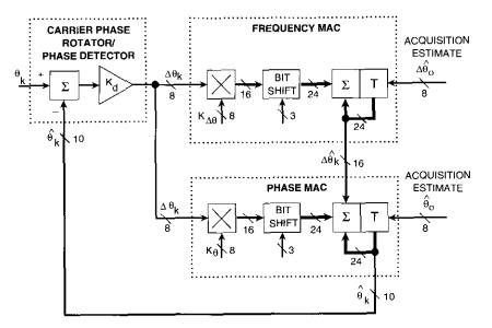
Figure 13. Carrier Phase Tracking Loop Model
