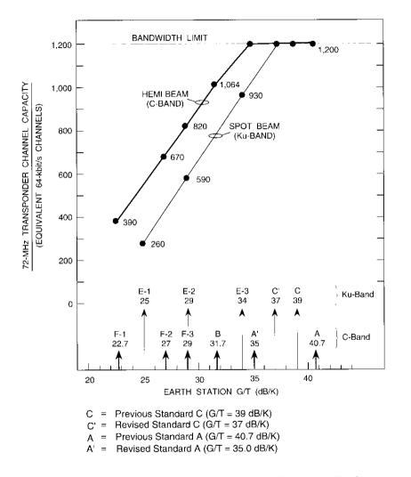
Figure 4. INTELSAT VI 72-MHz Transponder Capacity vs Earth Station G/T (Using digital IDR carriers with rate 3/4 FEC)
