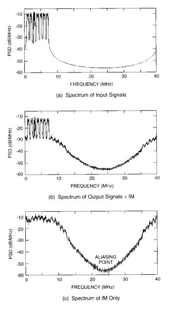
Figure 8. Picket Fence Frequency Plan: Equal Size and Equal Spacing
