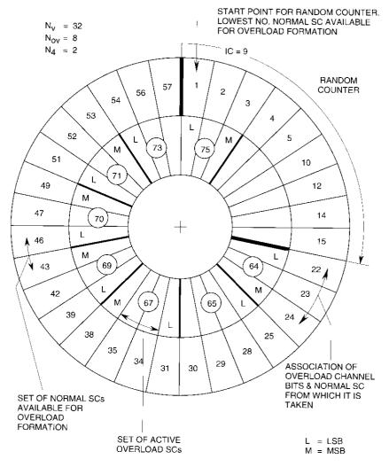
Figure 9. Selection of SCs for Bit Stealing
