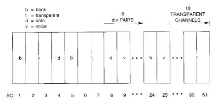
Figure 7. Bearer Configuration for Assignment Example
