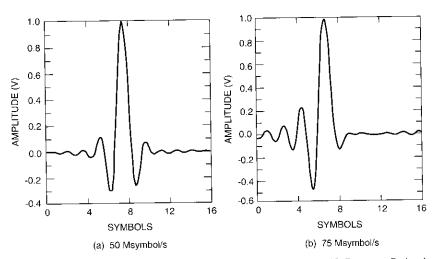
Figure 4. Predistorted Transmit Impulse Responses for a 40-Percent Raised Cosine Channel
