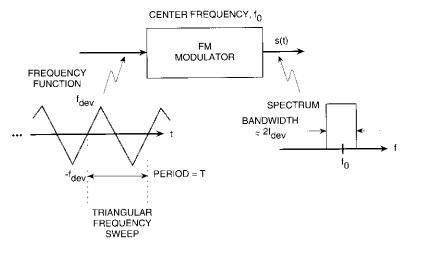
(a) Signal Generator Module for Energy-Dispersed CW
