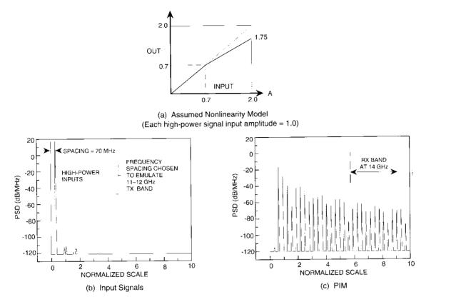
Figure 11. Effect of Varying Two-Section Nonlinearity Model (from Figure 10) to Observe Changes in PIM
