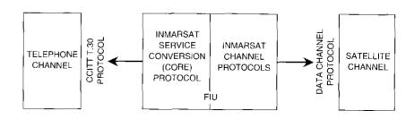
Figure 4. Block Diagram of FIU Protocol Partitioning
