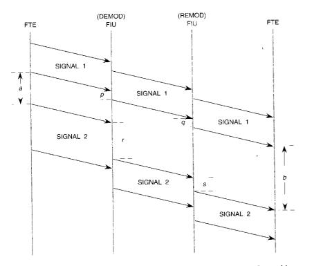
Figure 6. Example of Temporal Distortion at Destination FTE Caused by Detection, Demodulation, and Remodulation Processes
