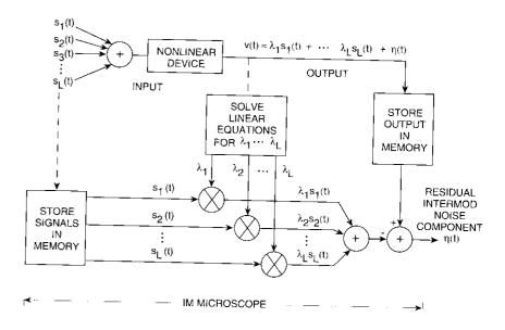
Figure 1. Equivalent Gain and Residual Noise Model Forming the Basis of the IM Microscope
