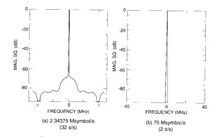
Figure 26. AGC Tracking Loop Output Phase Noise
