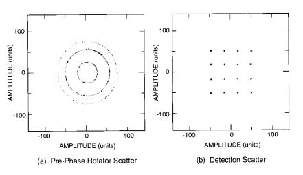
Figure 20. 16-QAM Demodulator Scatter Diagrams
