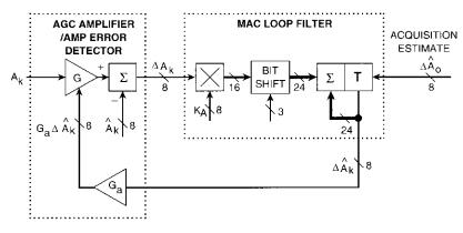
Figure 11. AGC Tracking Loop Model
