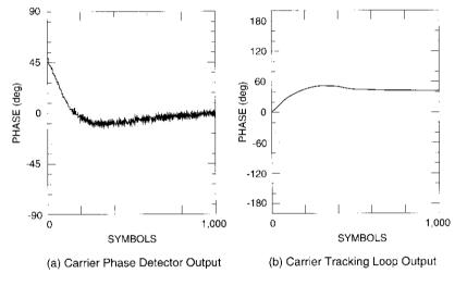
Figure 25. Carrier Phase Tracking Loop Transients
