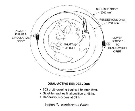
In addition to lowering INTELSAT 603's orbit, it was also planned to reduce its spin speed from about 15 rpm to 0.65 rpm in preparation for capture by the astronauts. These maneuvers, along with any required attitude reorientations and nutation damping, were to take place after CBST, about 6 hours before *Endeavour's* final approach.
