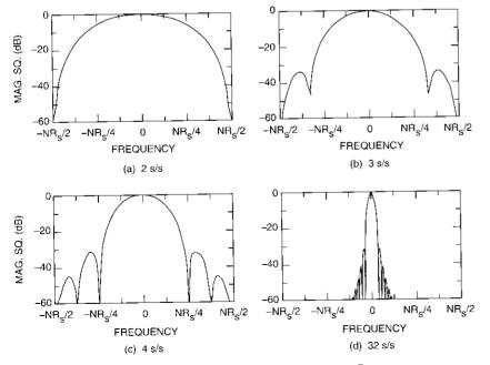
Figure 8. PA Receive Data Filter Frequency Response
