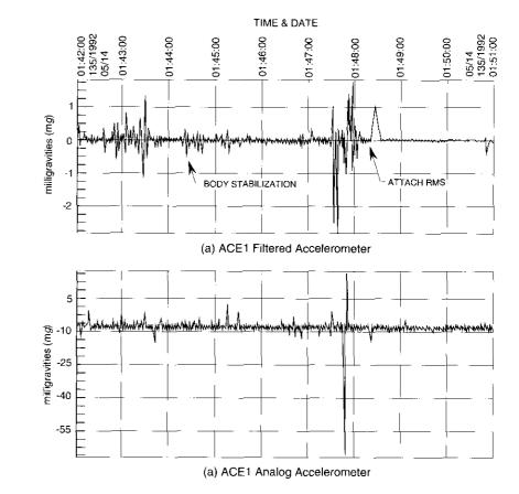
Figure 10. Accelerometer Signal: RMS Attachment
