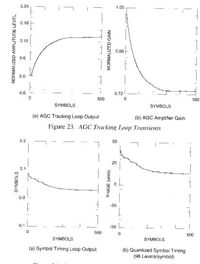
Figure 24. Symbol Timing Tracking Loop Transients
