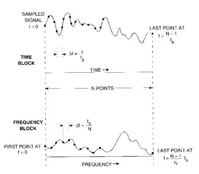
Figure 2. Time and Frequency Windows of Data Blocks With Discrete Fourier Transform
