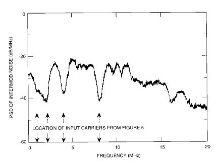
Figure 6. IM-Only Spectrum With 3rd-Order IM-Free Carrier Plan
