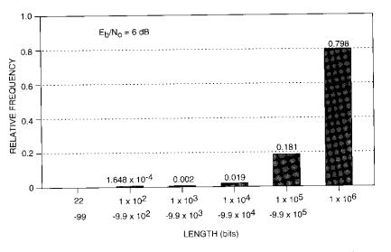
Figure 12. Relative Frequency of Length of Error-Free Interval
