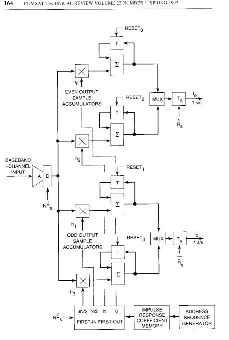
Figure 6. Dual Overlapping PA Receive Data Filter
