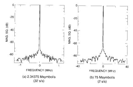
Figure 27. Carrier Phase Tracking Loop Output Phase Noise
