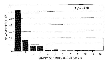
Figure 11. Relative Frequency of Contiguous Error Bits Within a Burst
