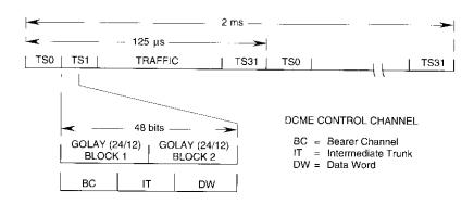
Figure 13. INTELSAT IESS-501 Frame Structure
