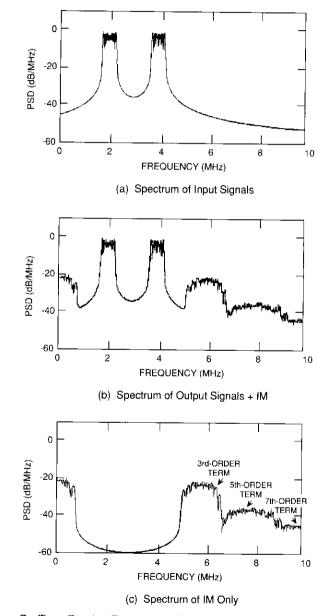
Figure 7. Two-Carrier Frequency Plan Showing IM Generation Out-of-Band
