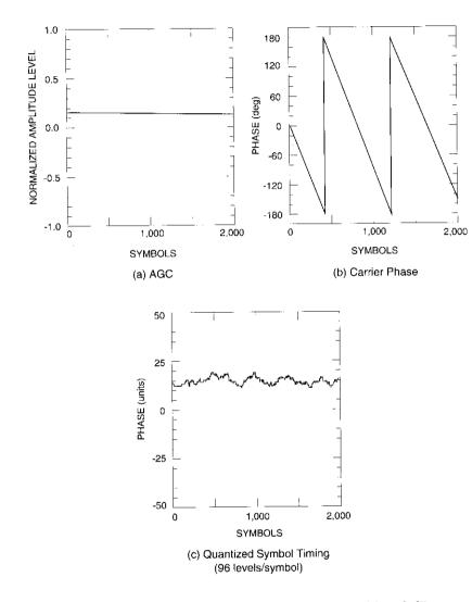
Figure 22. Tracking Loop Output Estimates at  $E_b/N_o = 0 \ dB$
