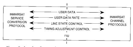
Figure 8. Interface Between Inmarsat Service Conversion and Inmarsat Channel Protocols
