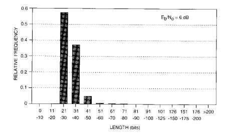
Figure 10. Relative Frequency of Length of Error Event (Burst)
