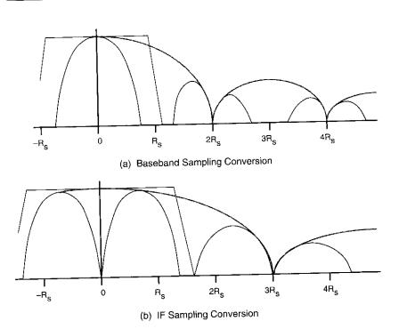
Figure 1. Modulator D/A Output Spectra
