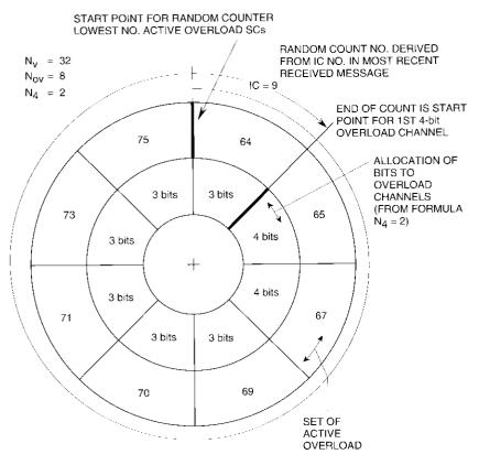
Figure 8. Selection of 3/4-bit Mode of Overload SCs
